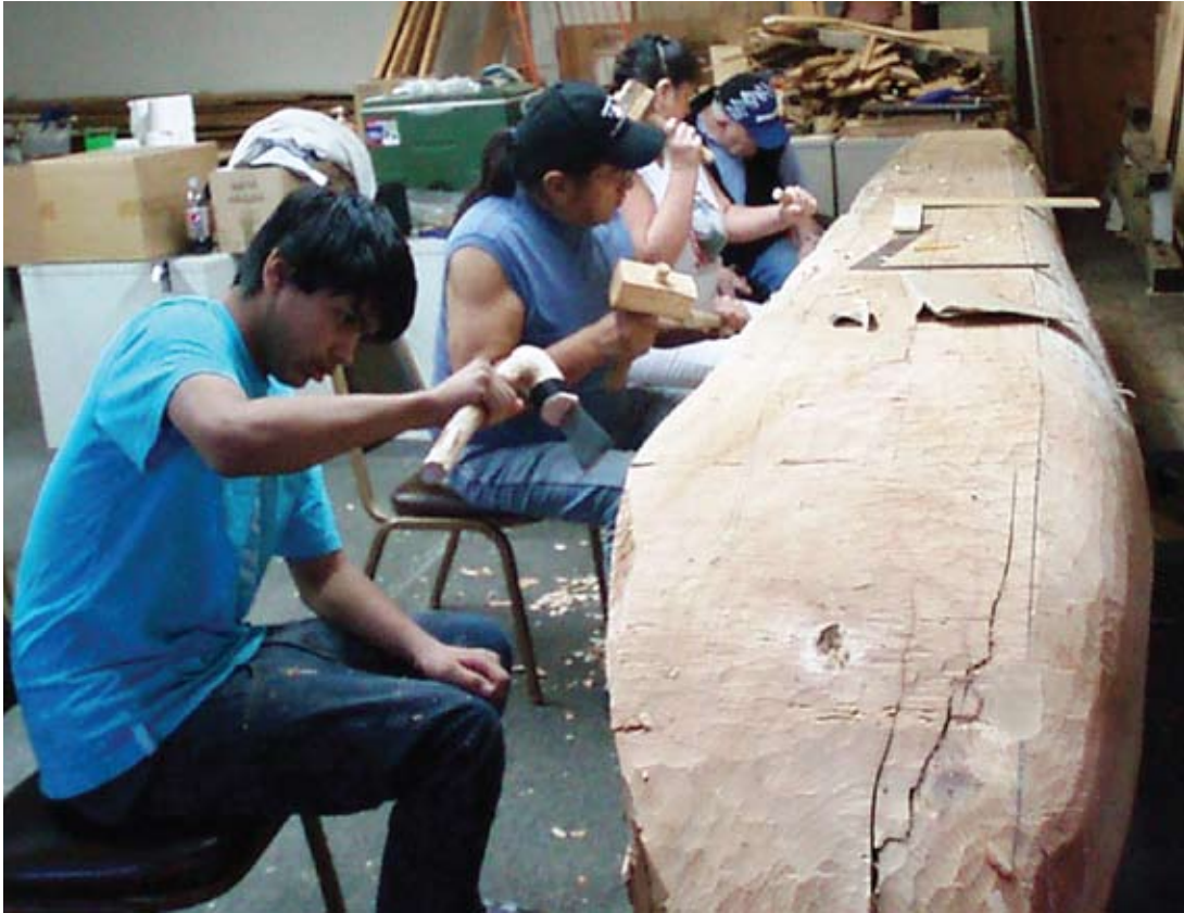
The dugout river canoe has been moved inside of the wood shop. The phase of carving the bottom of the canoe is almost finished. Pictured are (L-R) Antonio Sanchez, Sid Smith, Jodie Smith and John Penberth. Photo by Master Carver Dave Wilson
